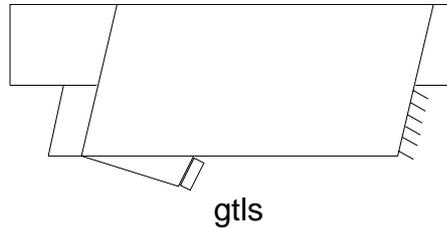
Any daylight remaining can shine into the top of the prism and light the phosphor of the gtls so assisting day/night takeover.
