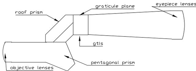
The target scene is focussed by the objective lenses (diameter 12 mm) onto the graticule plane via pentagonal and roof prisms which invert it; the eyepiece lenses (diameter 17 mm) focus it for the eye, putting it the right way up. The eye distance is 60 mm.
