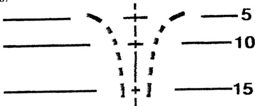
This is a graticule we designed to be used for firing the Vamma 155mm medium gun directly at moving targets: very simple, range in hundreds of metres, a boresight mark and leads shown by the breaks in the lines. A similar graticule is used in our RC-12 sight on the UK LAW 80.
