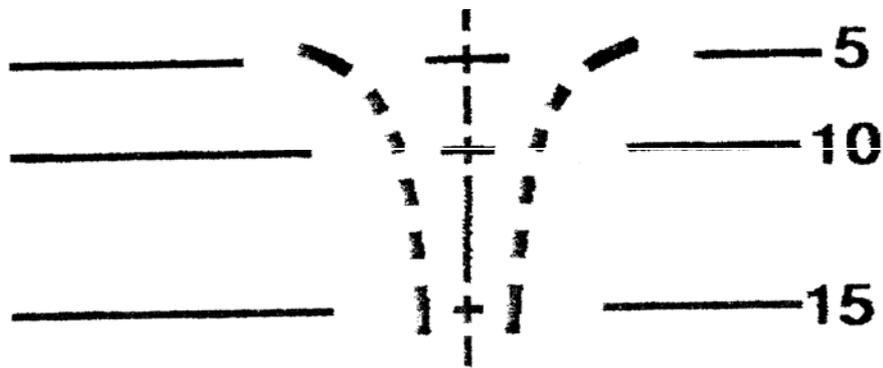
But we found during the LAW 80 sight research programme that stadia range estimation was only good to about 20%. You can use a laser rangefinder to advantage, either for making a range card, or during the engagement. The Ring Sights can have a pre-aligned dovetail for the lrf.
