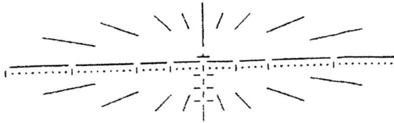
Same old boresight mark for 400 metres so the bullet strike is central at this range on the solid horizontal line. For 500 metres the dotted line is used and for greater ranges the lines below. Lead is more complicated when shooting sideways as aim off is required for helicopter movement: the bullets start with a forward velocity which is gradually lost by air resistance
