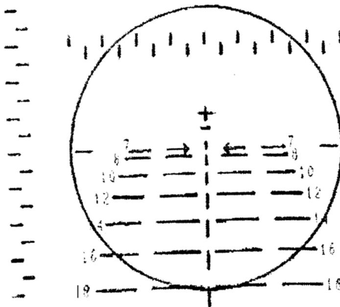
One of the problems is range estimation. Stadia lines can be added to help, as in this graticule for the ASP-30, where the tank fills the gap between the curved lines.
