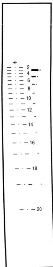
Elevations every 100 metres, even ones numbered. The drift on this weapon is considerable so you can see that it is allowed for by the aiming points being placed laterally to suit.
