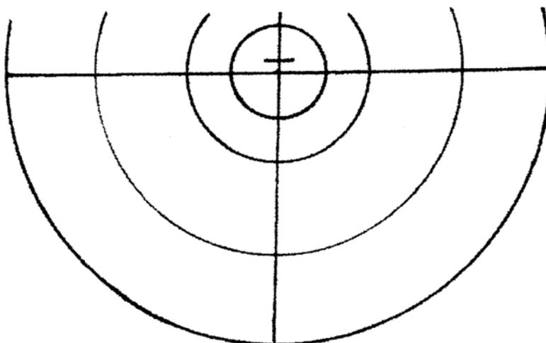
In this simple pattern the circles are at radii defined in mils: actually diameters of 25, 50, 100 and 150 mils. The gunner has to learn how to relate these to target crossing speeds so that he can choose the correct place on the graticule to ensure that the target arrives at the centre of the cartwheel when the bullets get there. It all depends on the time of flight to the range at which the target is to be hit. I will return to this later.
