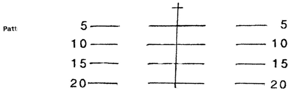
This is for the GPMG with an impact range of 700 metres, target height 100 metres and target speeds of 100, 200 and 300 metres per second. The radial lines are to help him getting the target flying towards the centre of the graticule (where the bullets will be).
